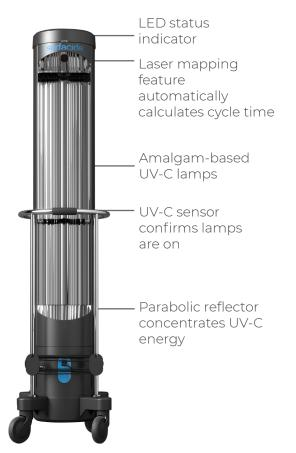
After the standard terminal cleaning process, position the Surfacide Helios UV-C System into the space and position the three robots in a triangular configuration.
