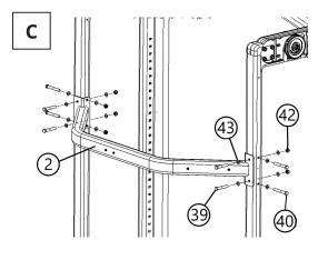
Place the **Pull-up Crossbar (3)** in position between the two main frames and insert four **M10x75mm Hex Bolts (39)** with **M10 Flat Washers (43)** through each main frame. Place **M10 Flat Washers (43)** and **M10 Locknuts (42)** onto the bolts. *DO NOT TIGHTEN THE HARDWARE AT THIS TIME.*
