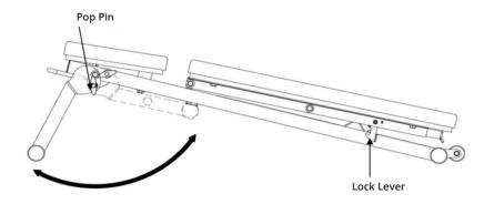
Pull pop pin to unfold or fold leg. Make sure hands are clear of pivot area. Make sure pop pin is fully engaged in locking holes after each adjustment.
