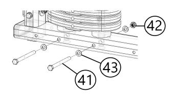
**A**. Route the cable as shown. Remove the pulley from the **Weight Stack Pulley (14)** assembly in order to route the cable into it, leave the hardware loose.
