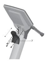
INSTALLING THE 550ETe2 CONSOLE— CONSOLE COVER.
