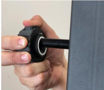
4. Once the knob is against the rack, release the button and turn the knob to tighten it.
