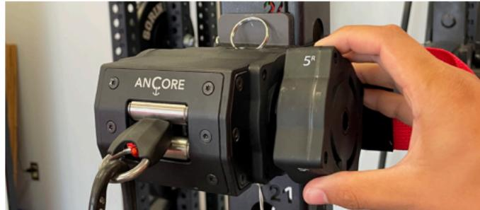
2. Start by placing the resistance plate at a 45 degree angle against the side of the base. Turn the plate quarter turn back and then rotate the plate toward you while placing light pressure to the center of the Trainer. When the plate is attached, there should be no visible space between plate and the base. Repeat for up to three resistance plates on each side of the base.
