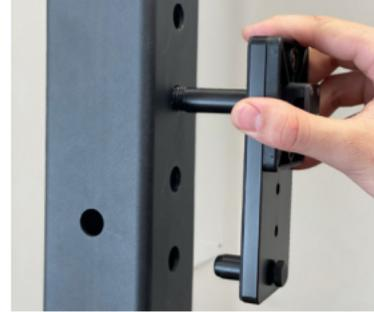
3. Take the knob, depress the button, slide the knob down the threaded shaft until the white ring rubs against the rack post.
